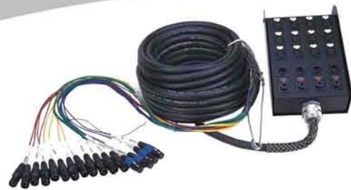
• AP-SC2445 > 16 channel stage box > Box end: 12xlr female+4xlr male with 4 1/4trs parallel. > Span end:12xlr male+4xlr female > Balanced cable available with different length
